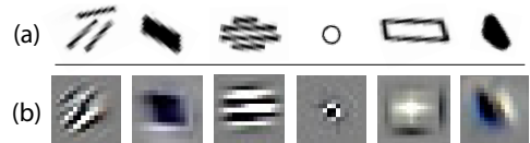
Figure 1: (a) : “Tokens” from Fig. 2-4 of Vision by D. Marr [1]. These idealized local groupings are proposed as an intermediate level of representation in Marr’s primal sketch theory. (b) : Selected filters from the 3rd layer of our hierarchical model, trained in an unsupervised fashion on real-world images using convolutional sparse image decomposition.
